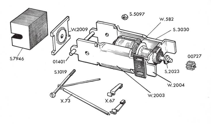
W.582 Armature Top Pole Piece with Diaphragm W.2003 Front Plate and Bearing W.2004 Back Plate and Bearing W.2009 Carbon Brush X.67 Diaphragm and Eyelet (Shown as part of W.2003) X.69 Brush Spring and Insulator X.73 Magnet Screw S.1019 S.2023 Thrust Bush Bottom Pole Piece 5.3030 8 BA Nut 5.5097 Magnet 5.7946 00727 Pinion
